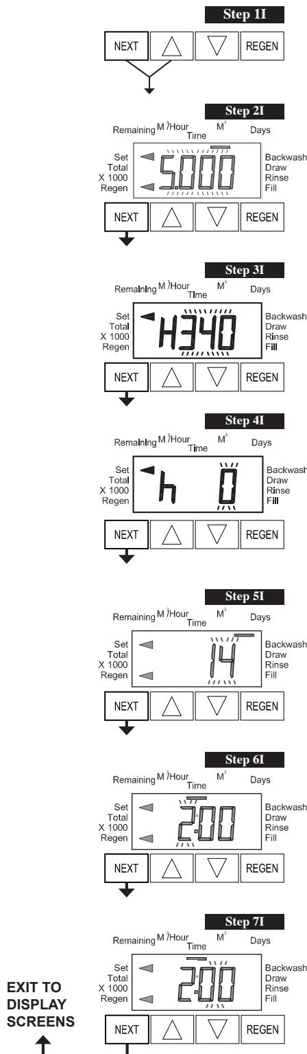
**Step 1I** - To enter Installer Display press NEXT and ▲ simultaneously for 5 seconds and release.
