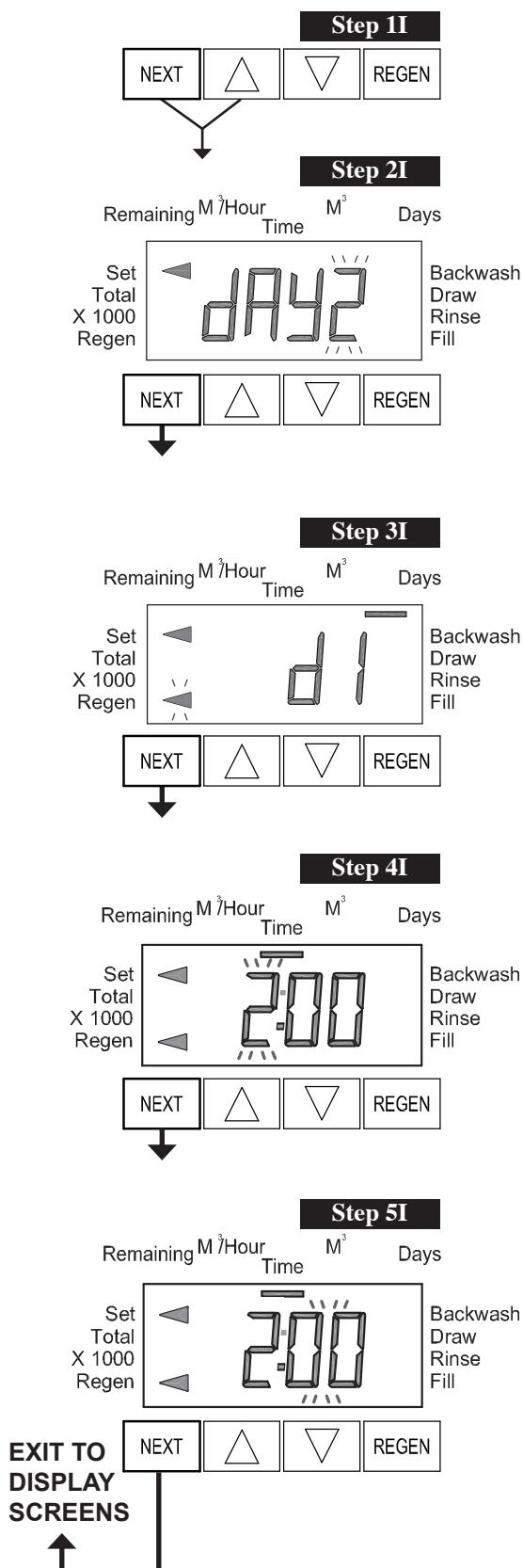
**Step 1I** - To enter Installer Display press NEXT and ▲ simultaneously for 5 seconds and release.
