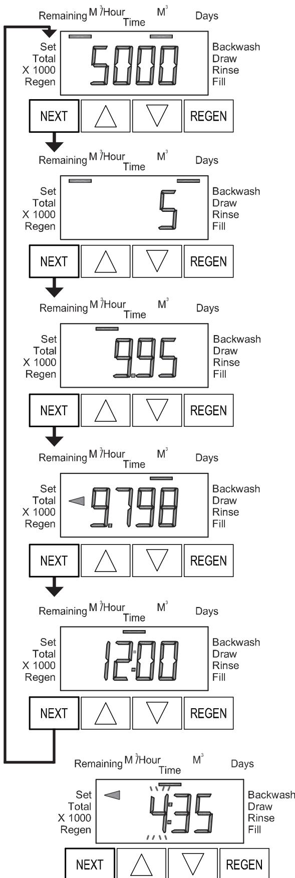
When the system is operating, one of five displays may be shown. Pressing NEXT will alternate between the displays shown below.
