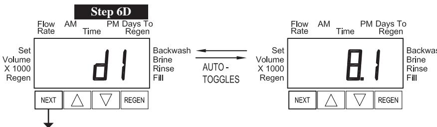
**Step 6D** - Display shows the daily voltage level of the battery pack. The first display is the day and the second display is the voltage. The voltage is recorded at midnight. The number of days ranges from 1 to 127. Press NEXT to go to Step 7D. Press REGEN to return to previous step.
