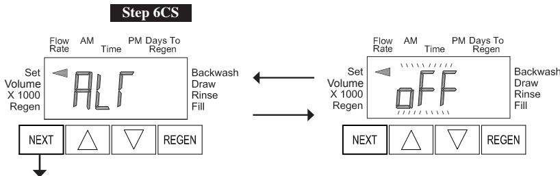
**Step 6CS** – Allows selection of one of the following using the ▲ or ▼ buttons:
