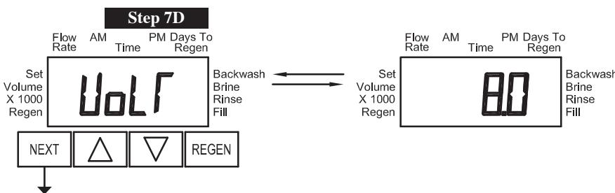
**Step 7D** - Display shows the latest measured voltage of the battery pack. Pressing and holding the ▲ and ▽ buttons simultaneously for approximately 5 seconds will initiate a test of voltage. (Normally this test is automatically conducted at 12:00 am daily.)
