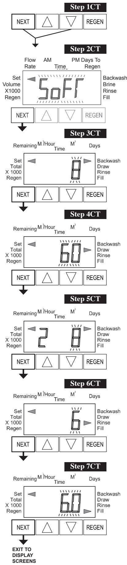
**Step 1CT** - Press NEXT and ▼ simultaneously for 5 seconds and release. If screen in Step 2CT does not appear, the lock on the valve is activated. To unlock press ▼, NEXT, REGEN, ▲ in sequence, then press NEXT and ▼ simultaneously for 5 seconds and release.
