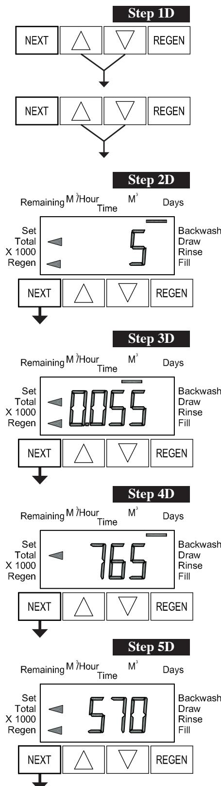
**Step 1D** - Press and simultaneously for 5 seconds and release. Then press and simultaneously for 3 seconds and release. If screen in Step 2D does not appear the lock on the valve is activated. To unlock press , NEXT, REGEN, in sequence, then press and simultaneously for 5 seconds and release. Then press and simultaneously for 3 seconds and release.
