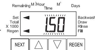
**Step 3CT** - Adjust the length of the backwash from 1-95 minutes using ▲ or ▼.
