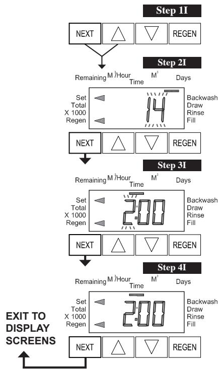
**Step 1I** - To enter Installer Display press the NEXT and ▲ simultaneously for five seconds and release.
