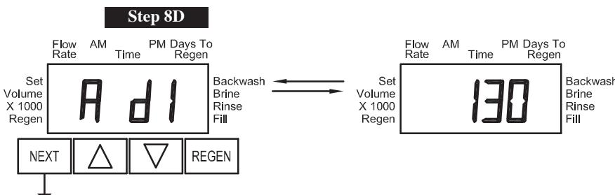
**Step 8D** - Display shows the daily measured mA/hr charge of the battery pack. An active Regen Arrow indicates that a regeneration cycle occurred on that day.
